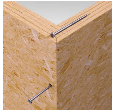
90° inside wall corner
